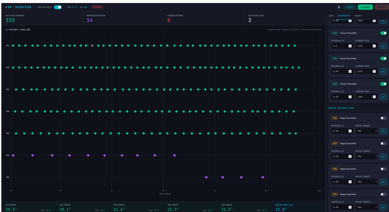
Figure 5.104 Spoofing scenario as visualised through the RF fingerprinting monitoring dashboard
