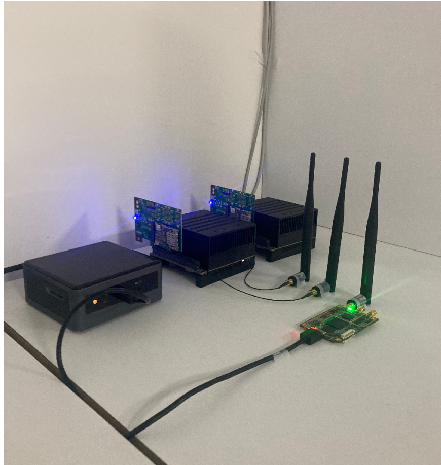
Figure A.1: The receiver array setup consisting of synchronized XTRX and B200 Mini SDRs.
