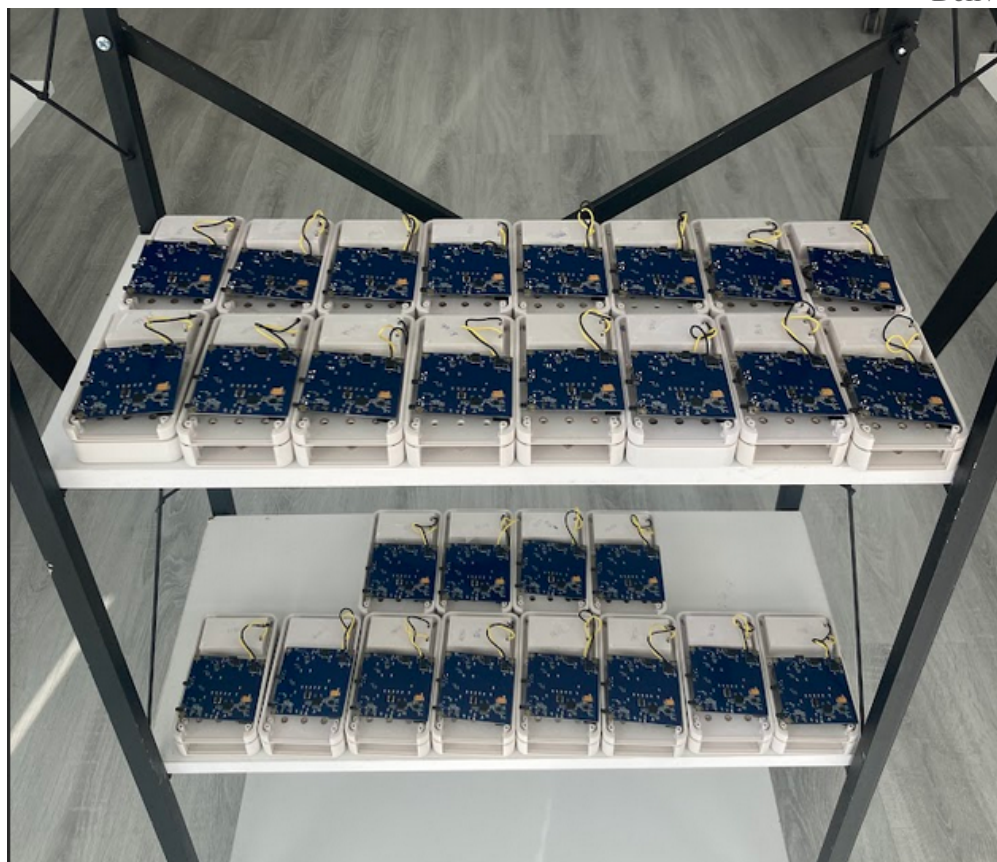
Figure A.2: The set of 28 identical, custom-manufactured IoT transmitters used to evaluate the RF fingerprinting migration.
