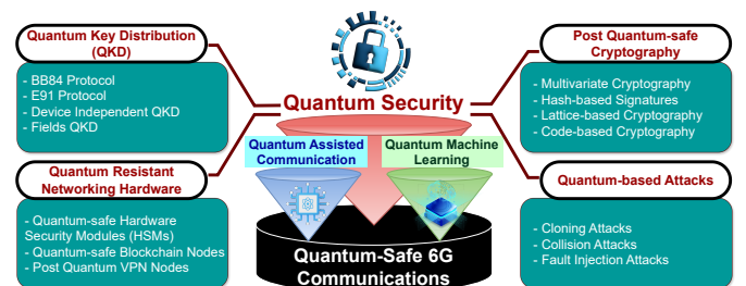
Fig. 4: Quantum-Safe 6G Communications. Different types of post-quantum cryptography algorithms and approaches have so far been developed to counter the threat posed by quantum computers to classical encryption
