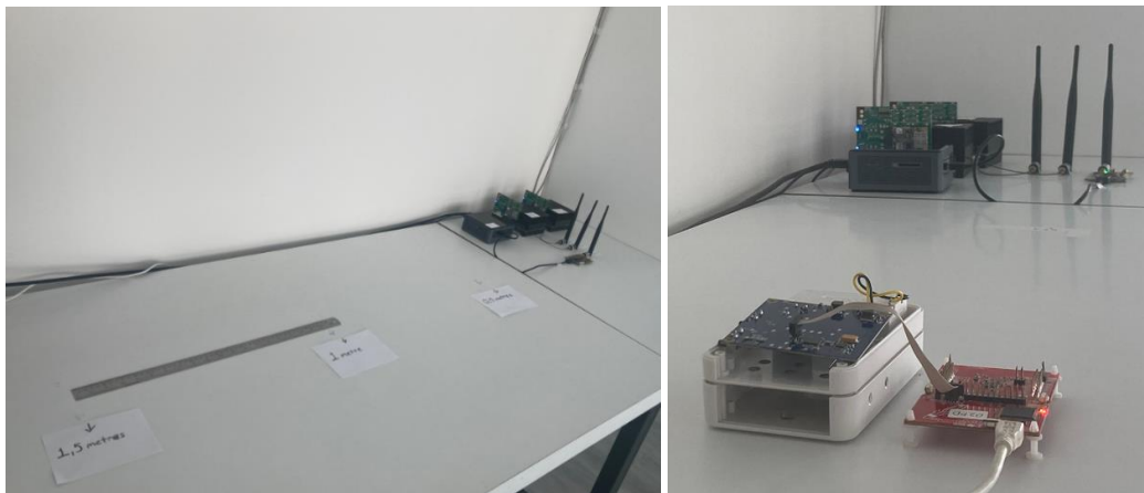
Figure 3-3: Data Collection Setup & Transmitter and Receiver while on operate at 1 meter
