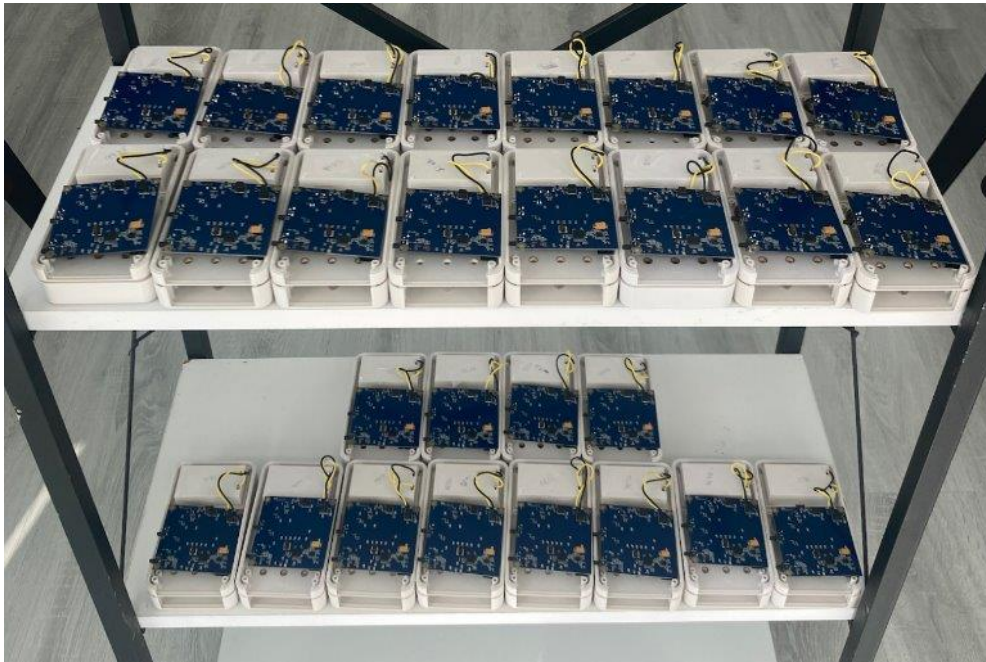
Figure 3-2: TI13XX-based designed IoT sensors used in RF Fingerprinting Migration Dataset
